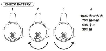
**Colored leds:** A colored led seen in the lens, indicates the battery level each time the light is switched off.
